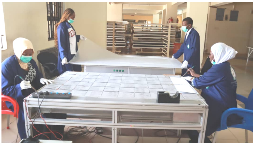
Stringing and soldering of solar cells at NASENI Solar Energy Limited, Karshi, Abuja.
